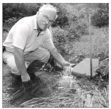
Bruce Smith, co-ordinator with the Winter River-Tracadie Bay Watershed Association, uses a small V-shaped dam to measure the depth and calculate the flow of streams and springs in the watershed. July's dry weather has taken a toll on the flow.
