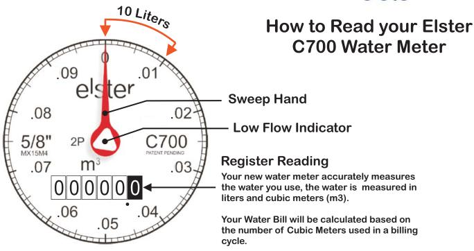
As water passes through the meter the "Sweep Hand" moves around the dial, each complete revolution of the dial equals 100 liters of water.
