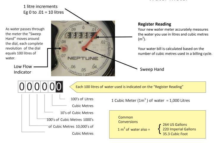
The triangular shaped "Low Flow Indicator" to the left of the register dial will move when even the smallest amount of water is passing through the meter. You should use the "low flow indicator" periodically to check for leaks in your property.
